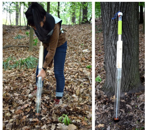
Figure 4: Spore Stepper is a walking stick that can also be used to collect soil samples.
